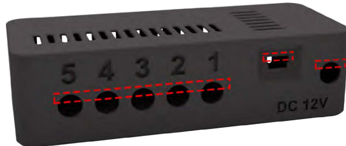
Fig. 1: Areas that may require post-print clean-up to remove hanging material.
