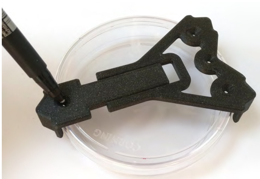
Fig. 15: Transferring hole locations to a 10 cm petri lid.
